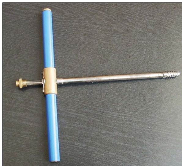
Fig. 4. Appearance of incremental Pressler drill (Fig. K. Krajewski).
