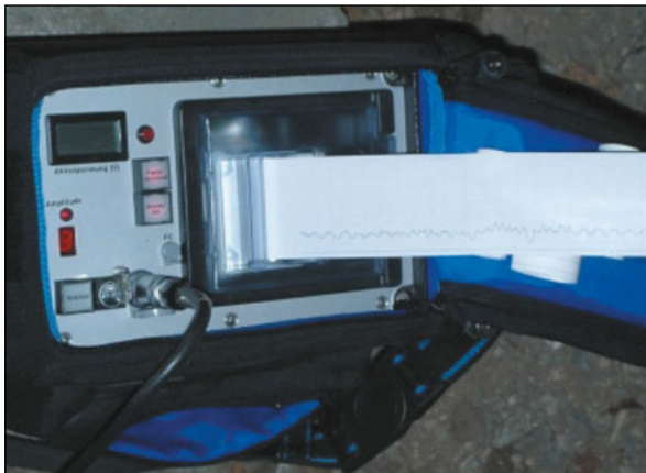
Fig. 6. Example of visualization of the results of wood drilling with a Resistograph:
