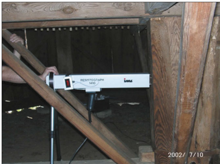
Fig. 5. Testing the structure of a historic treadmill at the Museum of Agriculture in Ciechanowicz, (fig. K. Krajewski).
