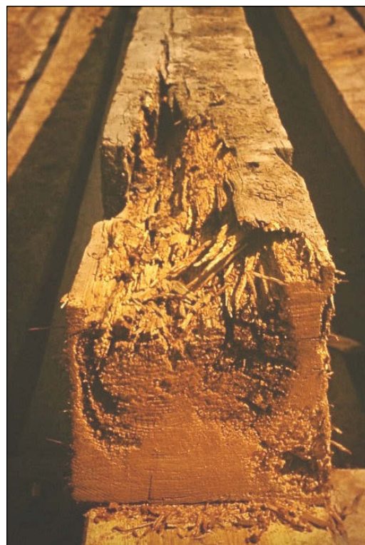
Fig. 3. An example of a fragment of wood with internal decomposition, (Fig. collections of the Wood Protection Department at Warsaw University of Life Sciences).
