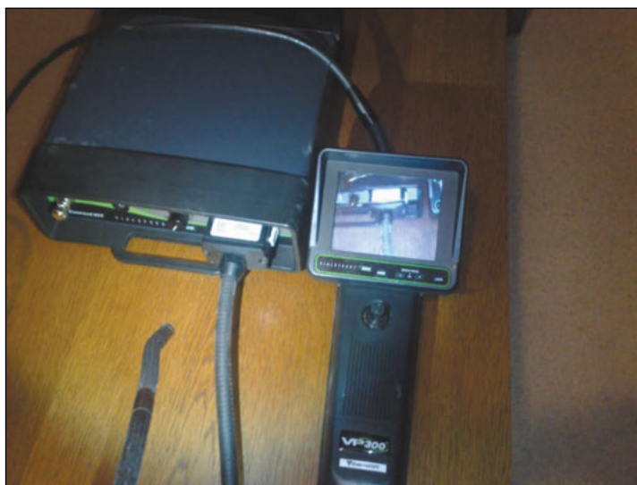
Fig. 2. The endoscope also referred to as an inspection camera, (Fig. K. Krajewski).
